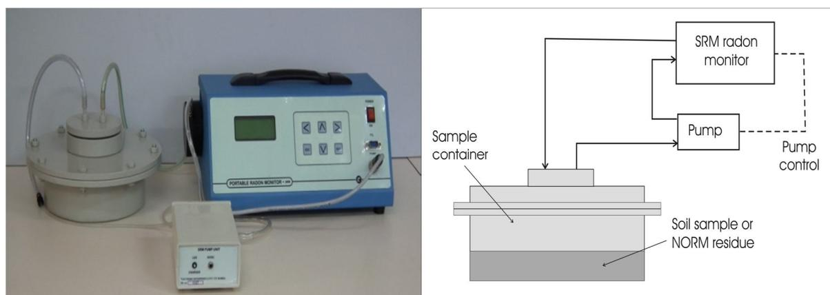
**Fig.1:** Photograph and schematic diagram of the radon/thoron exhalation measurement set up
