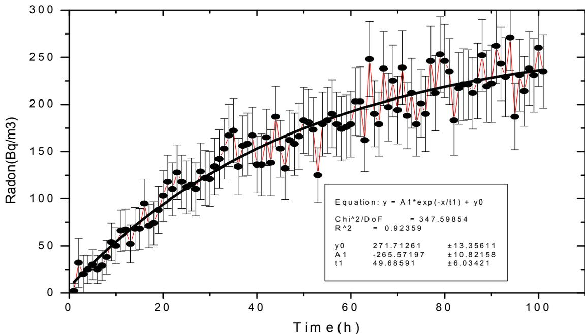
**Fig. 2:** Least square fitting of Eq. (2) to data plotted between radon concentrations in chamber with time
