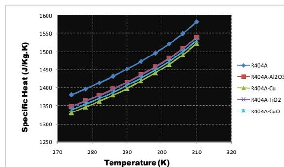
Fig.-3.4(a)-3.4(c) shows variation in Specific heat of nanorefrigerants with variation of temperature it was found that the specific heat variation of nanorefrigerant is increasing as temperature is increasing and also the similar to pure refrigerant as higher temperature High Specific heat and lower temperature low. But when we go for higher vol % concentration of nanoparticle specific heat will reduce.
