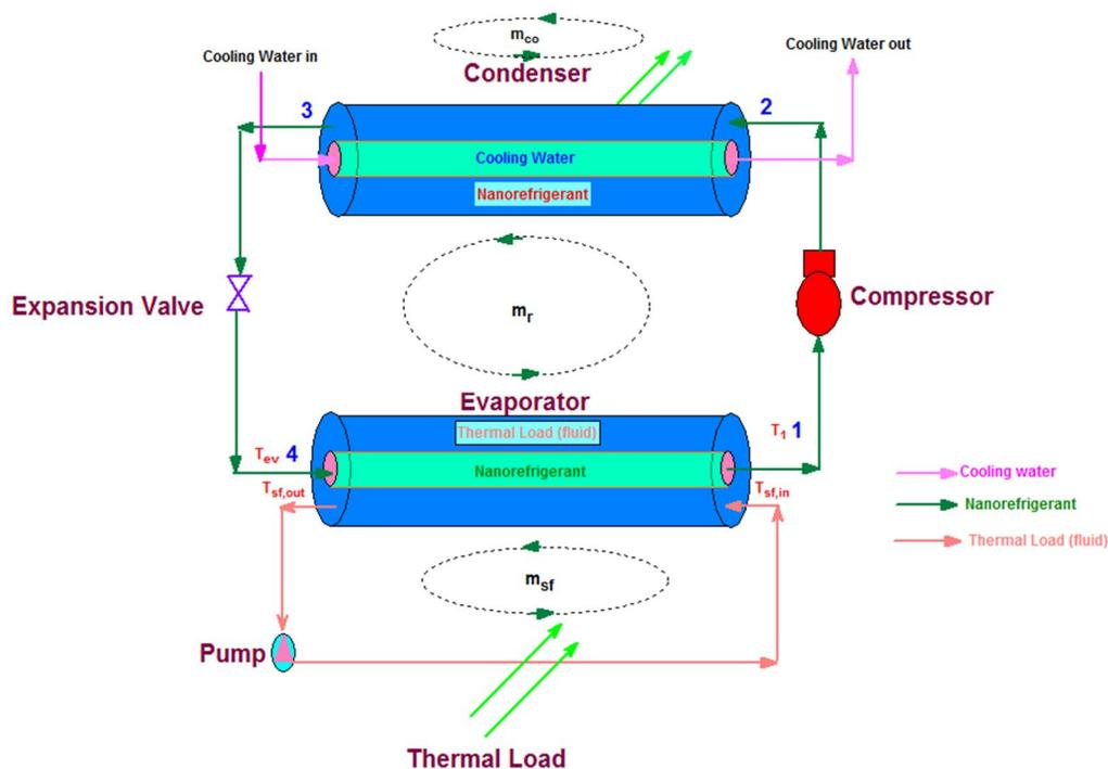
**Fig-1(b):** Experimental set of variable-speed vapour compression refrigeration systems
