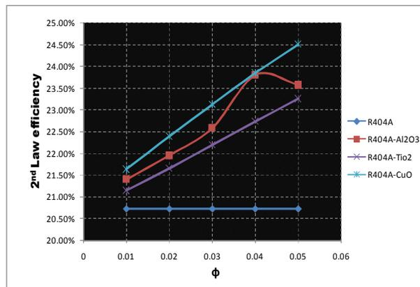
Fig 3.8(a)-3.8(c) showed the variation of exergetic efficiency (i.e. 2<sup>nd</sup> Law efficiency) with variation of ( $\phi$ ) and it was observed that as ( $\phi$ ) increases the exergetic efficiency is also increases and also it will increases by using nanorefrigerant.
