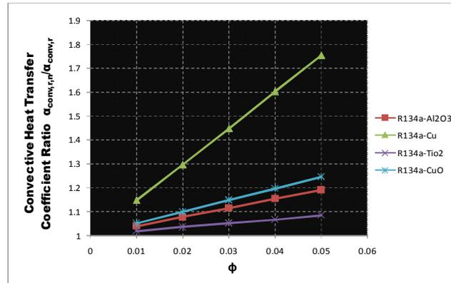
Fig 3.5(k) - 3.5(m) shows the convective heat transfer coefficient factor increases by increasing the concentration of nanoparticle. And copper nanoparticle based nanorefrigerant have highest convective heat transfer coefficient ratio than other particle its value ranges from 1 to 1.7.
