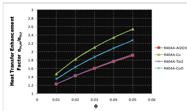
**Fig. 3.5(p):** Vol % concentration ( $\phi$ ) vs Heat transfer enhancement factor R407c with different nanoparticle
