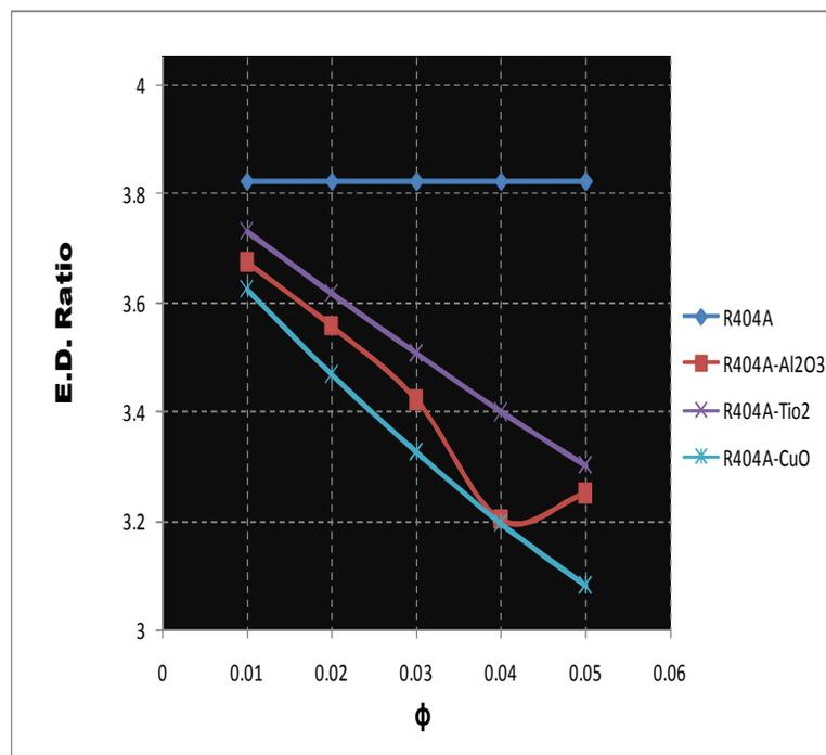
Fig 3.7(a)-3.7(c) shows the variation with of Exergy Destruction. Ratio (EDR) with variation of ( $\phi$ ) of ecofriendly refrigerants in the vapour compression refrigeration system (VCRS) and it was observed that exergy destruction ratio (EDR) is decreases as ( $\phi$ ) increases and will reduce by using nanofluid (nanoparticle based nanorefrigerant)
