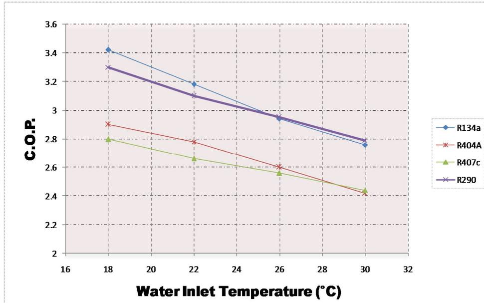
**Fig. 2(d):** COP vs. Brine inlet temperature of different refrigerants
