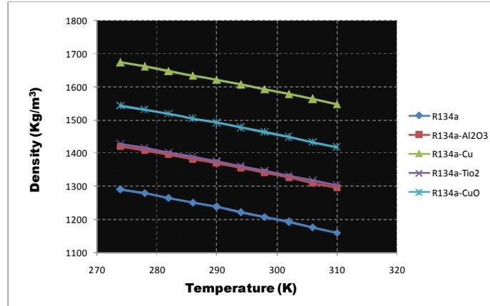
Fig. 3.2(b): Temperature vs Density of R404Aa with different nanoparticle
