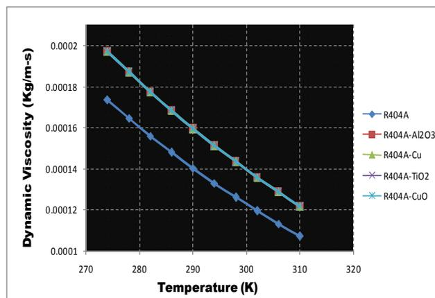
Fig. 3.3(a) to fig. 3.3(c) shows variation in Dynamic viscosity of nanorefrigerant subject to temperature variation. Fig shows that Dynamic viscosity variation of nanorefrigerant is similar to pure refrigerant as higher temperature low viscosity and lower temperature high.
