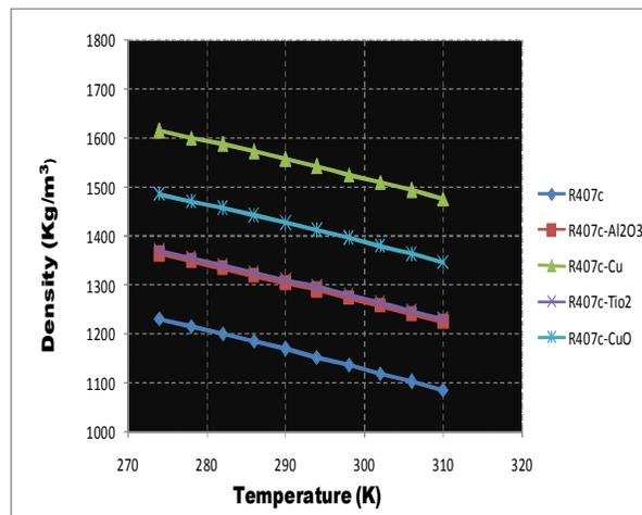
Fig. 3.2(a) -3.2(c) shows variation in density of nanorefrigerant subject to temperature variation. Fig shows that density variation of nanorefrigerant is similar to pure refrigerant as higher temperature low density and lower temperature high.
