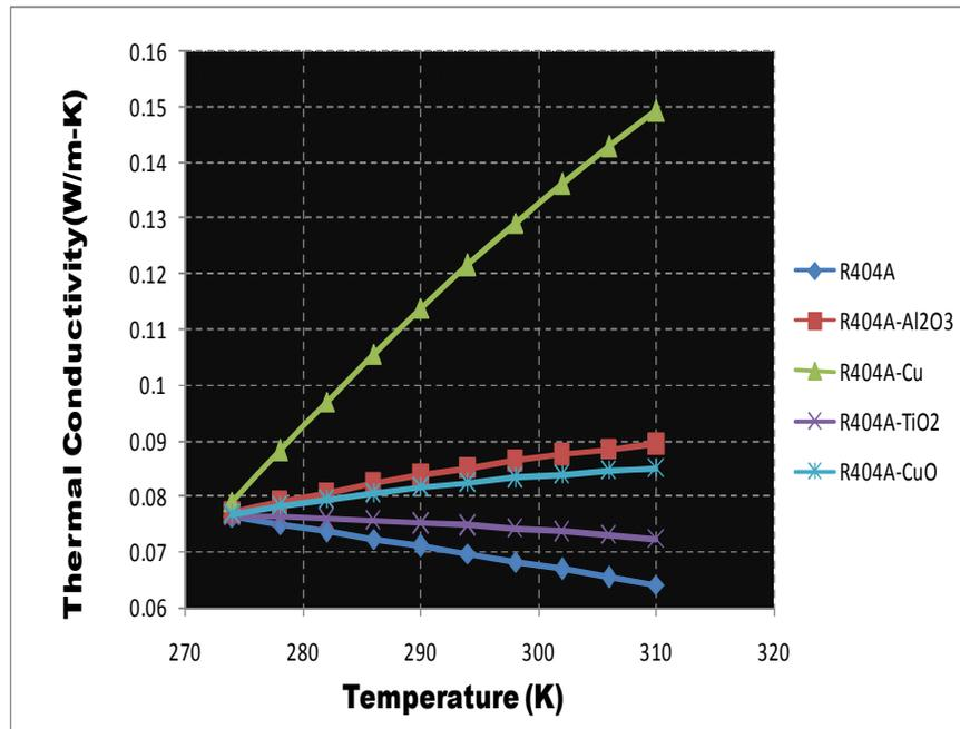
Fig. 3.1(a) -3.1(c) show the enhancement in thermal conductivity of pure when different kind of nanoparticle is suspended into the host refrigerant. The enhancement factor varies from 0.06 to 2 for different nanoparticle from the fig we can see that cu nanoparticle have more EF at higher temperature which value is approx 2.
