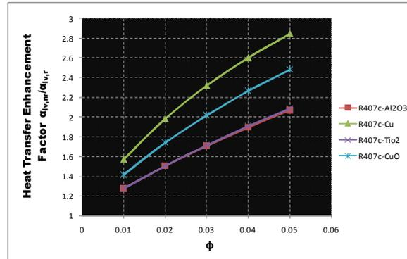
Fig.3. 5(n) -3.5(p) show the heat transfer enhancement factor of nanorefrigerant with different nanoparticle and it was observed that as Vol % concentration ( $\phi$ ) increases, the heat transfer enhancement is also increases and its value ranges from 1.2 to 3.2 and it was found that as for R134 a with cu nanoparticle have highest enhancement factor (EF ) approx 3.2 at 5 vol %.
