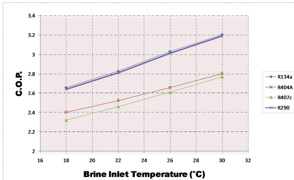
In Fig 2(d) the performance curve is shown between COP and Brine inlet temperature of different refrigerants. When brine inlet temperature 18 to 30 °C (66.67%) then change in COP for R134a is 20.46%, R404a is 17.15%, R407c is 18.47% and R290 is 20.54%.
