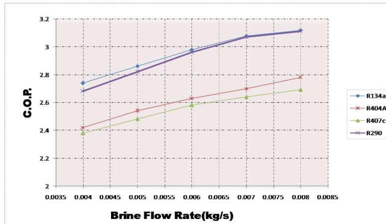
In Fig-2(a) the performance curve is shown between COP and Brine flow rate of different refrigerants. When brine mass flow rate 0.004 to 0.008 kg/s (100%) then change in COP for R134a is 14.10 %, R404a is 13.94%, R407c is 14.39% and R290 is 17.06%.
