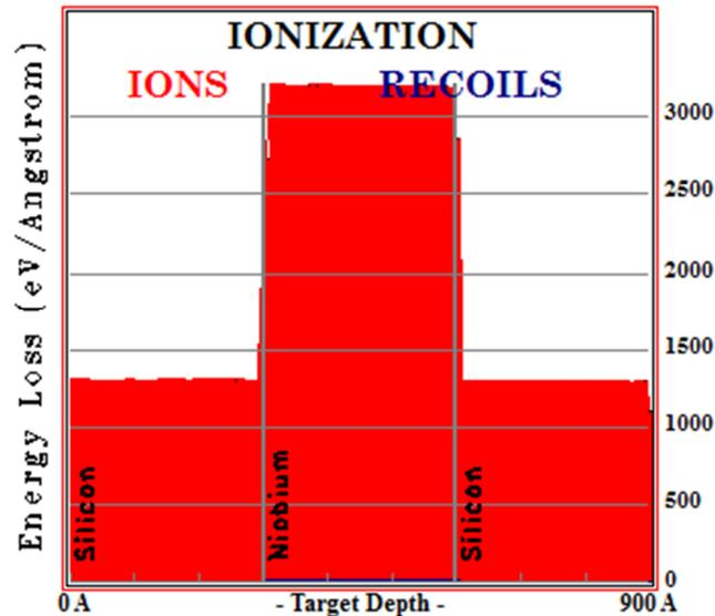
Fig. 1: Graphical representation of the Energy Loss as obtained by TRIM code
