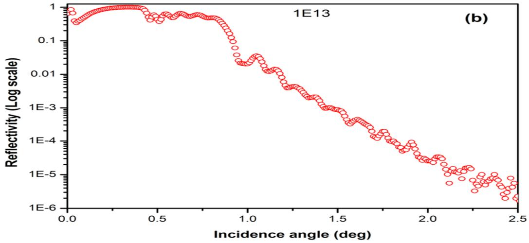
**Fig. 3(b):** Reflectivity curve of irradiated Si/Nb/Si thin film system at  $1 \times 10^{13}$  ions/cm<sup>2</sup>
