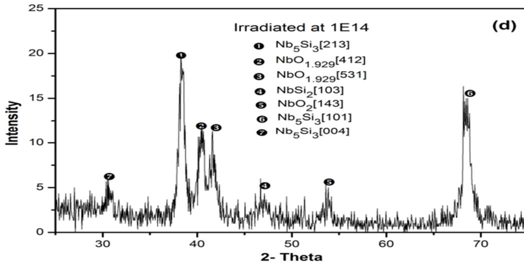
Fig. 2(d): GI-XRD curve of irradiated Si/Nb/Si thin film system at  $1 \times 10^{14}$  ions/cm<sup>2</sup>
