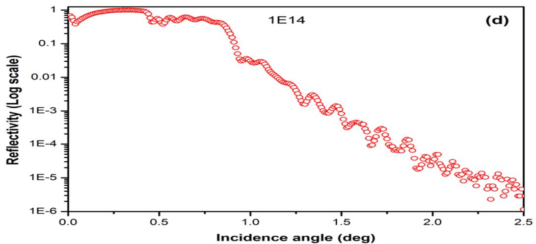
**Fig. 3(d):** Reflectivity curve of irradiated Si/Nb/Si thin film system at  $1 \times 10^{14}$  ions/cm<sup>2</sup>
