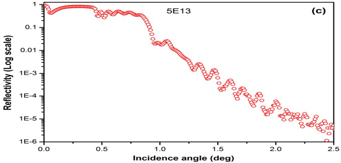
**Fig. 3(c):** Reflectivity curve of irradiated Si/Nb/Si thin film system at  $5 \times 10^{13}$  ions/cm<sup>2</sup>
