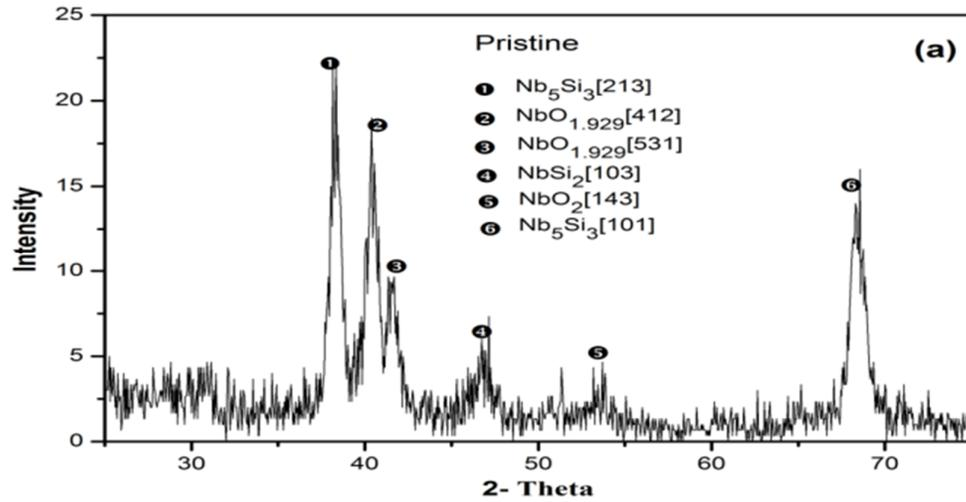
Fig. 2(a): GI-XRD curve of unirradiated Si/Nb/Si thin film system
