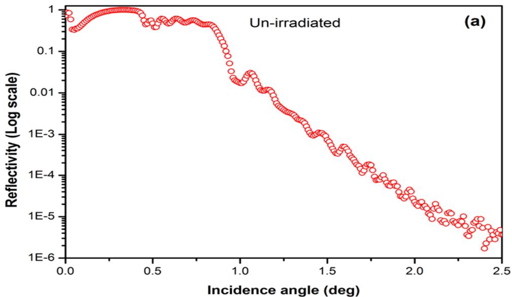
**Fig. 3(a):** Reflectivity curve of unirradiated Si/Nb/Si thin film system
