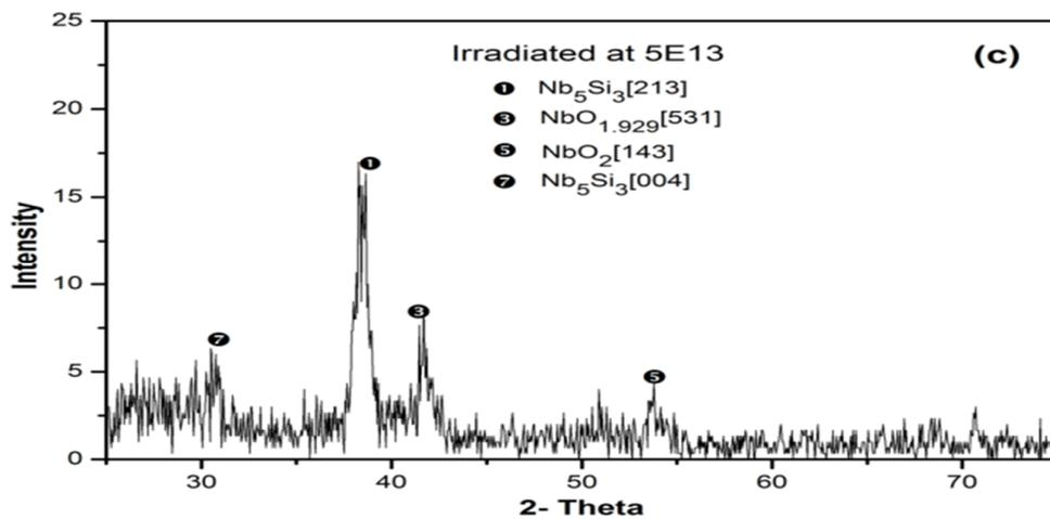
Fig. 2(c): GI-XRD curve of irradiated Si/Nb/Si thin film system at  $5 \times 10^{13}$  ions/cm<sup>2</sup>
