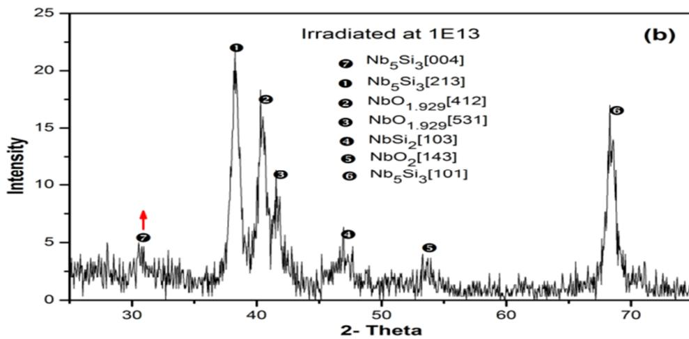
Fig. 2 (b): GI-XRD curve of irradiated Si/Nb/Si thin film system at  $1 \times 10^{13}$  ions/cm<sup>2</sup>
